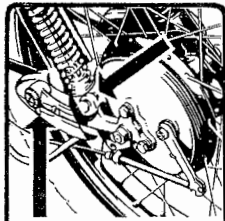
1 R. Swinging link &amp; Front fork spring bearing
